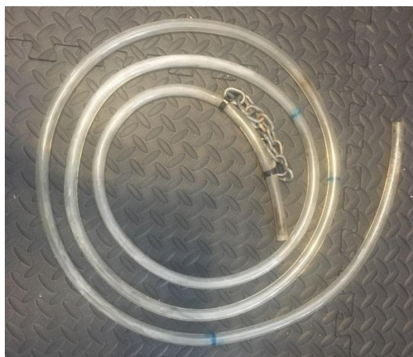
Figure 17. The 3-meter tube used for algae sampling.
