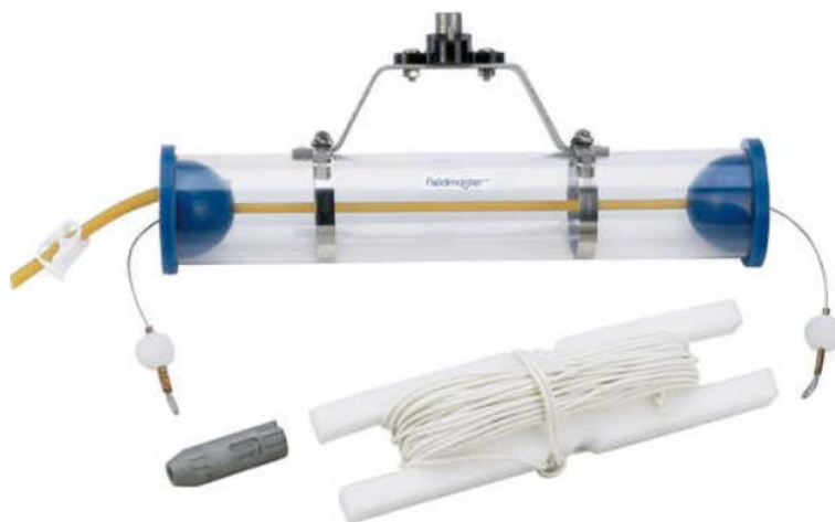
Figure 16. Van Dorn bottle for water quality sampling.
