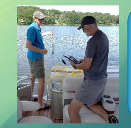
Dissolved Oxygen Monitor –It measures the temperature, dissolved oxygen and percent oxygen saturation at various depths.
