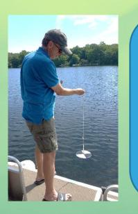
Secchi Disk – This measures the clarity of the water by lowering a black and white Secchi Disk into the water until it can no longer be seen
