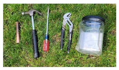
There are other totally acceptable ways to do it, but this is how I gathered the sample. All you need is a hammer, pliers, screwdriver, quart container and a 4"-5" length of pipe. Bang the pipe 4" into the ground with the hammer. Pull it out with the pliers and scrape the soil out of the pipe into a container with the screwdriver. Repeat in multiple locations of your lawn until you have a total of about a pint of soil. Try to spread out the locations
